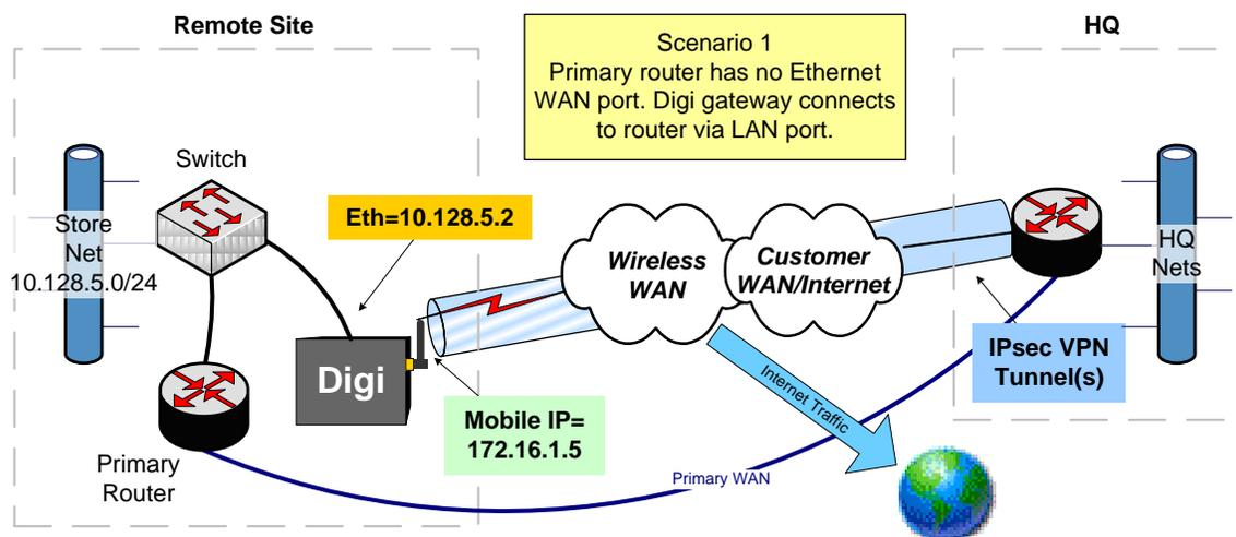
How it works: In most cases, the Primary Router will be configured with a floating static route using a higher metric, such as 256, pointing to the Digi gateway's Ethernet IP address (e.g., 10.128.5.2). In some cases, an intelligent layer 3 VLAN switch could handle the routing and failover (note the Digi gateway does not support VLAN itself).
