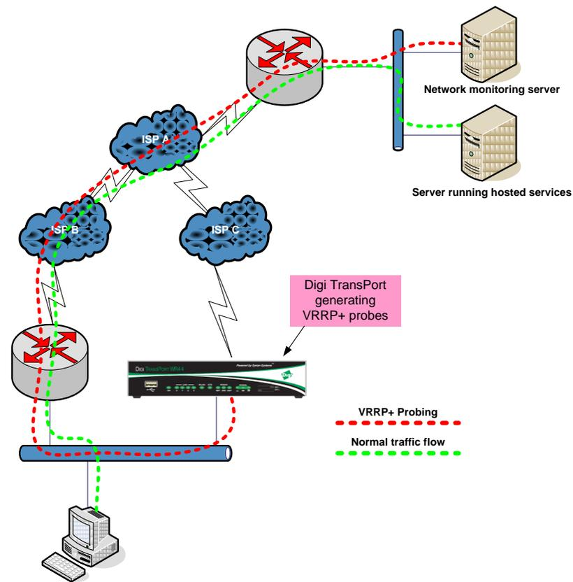
The diagram above shows the path of the VRRP+ probes sent from the Digi TransPort to a host on the remote network and the path of normal data traffic.
