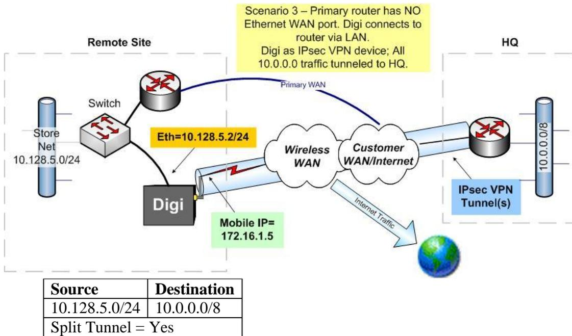
Why use this method? This is somewhat a compromise between the two approaches above. It still allows split tunneling but simplifies the VPN policy configuration and helps facilitate a “flat” network.
