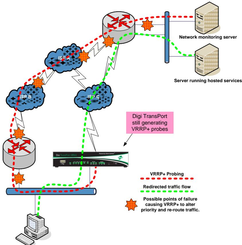
The above diagram shows the TransPort assuming the master router role while continuing to send probes.
